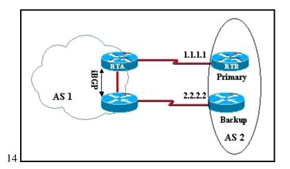
Assume all routers are running BGP sessions and both links are operational. Write the command set that would insure AS1 routers use link 1.1.1.1 for packet transmittal to AS2?
