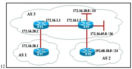
From the given configuration taken from RTA and graphic, which network will be filtered from being propagated to RTC from RTA?
