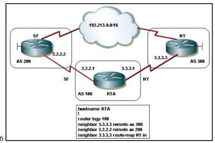
Refer to the diagram and configuration. RTA receives the prefix 192.213.0.0/16 from both providers SF and NY. Write out the route-map configurations for RTA that will set up NY as a primary link and SF as a backup link?
