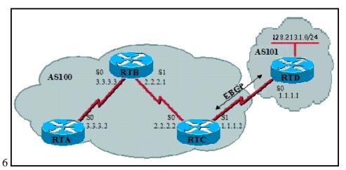
Given the above diagram, which address will RTB view as the next hop address to reach network 128.213.1.0/24?
